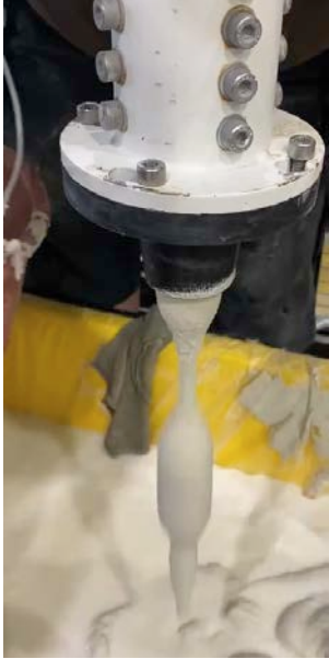
Fig. 38 The principle of the slugs test to determine the mortar's yield stress at the nozzle outlet.
