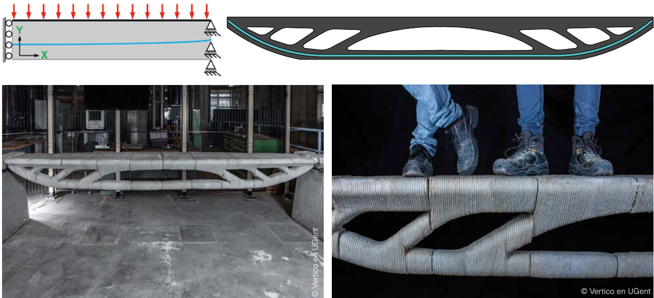
Fig. 17 Results of topology optimisation on a one-off, single-span girder under uniform load (top, [O1]) and 3D printing for the optimal footbridge (bottom).
