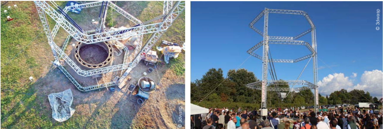
Fig. 45 3D printer Big Delta .
