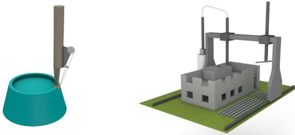
Fig. 4 The process of Contour Crafting (left) and the principle of building on a large scale using this process (right) [K1].
