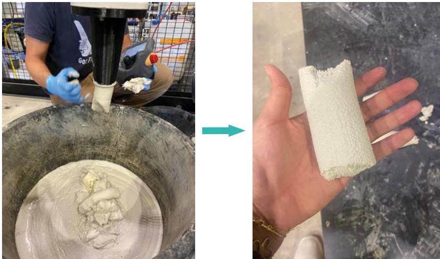
Fig. 37d 3D printing experiments conducted at Buildwise. Mixture considered too stiff (not extrudable).
