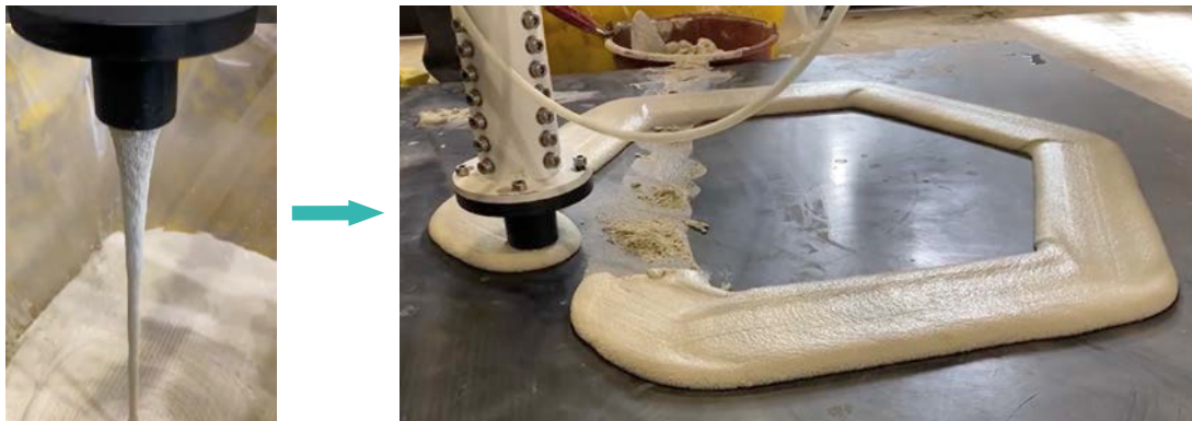
Fig. 37b 3D printing experiments conducted at Buildwise. Mixture considered too fluid (high slump, non-buildable mixture).
