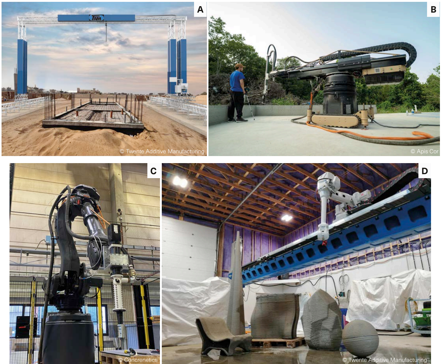
Fig. 6 Gantry system printer (A), lever printer (B), six-axis robotic arm printer (C) and nine-axis printer with robotic arm, mounted on a gantry (D).
