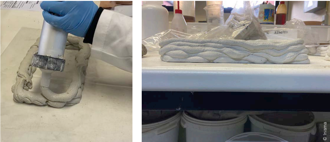
Fig. 39 Silicone gun used to test the extrudability of printable mixtures (left) and example of layers printed using this gun (right).
