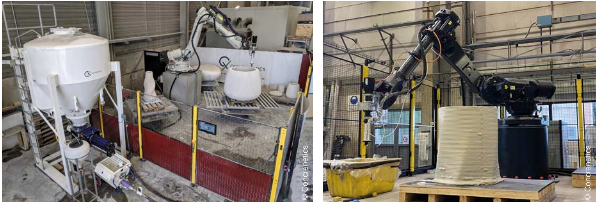
Fig. 42 One-X Industry system (left) and an element printed using this system at Buildwise (right).
