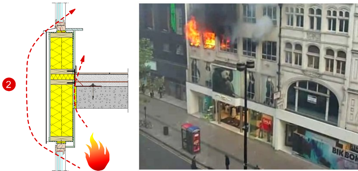
Figure 10 – Internal and external fire spread. Left: schematic drawing; right: flames coming out of a burning floor.
