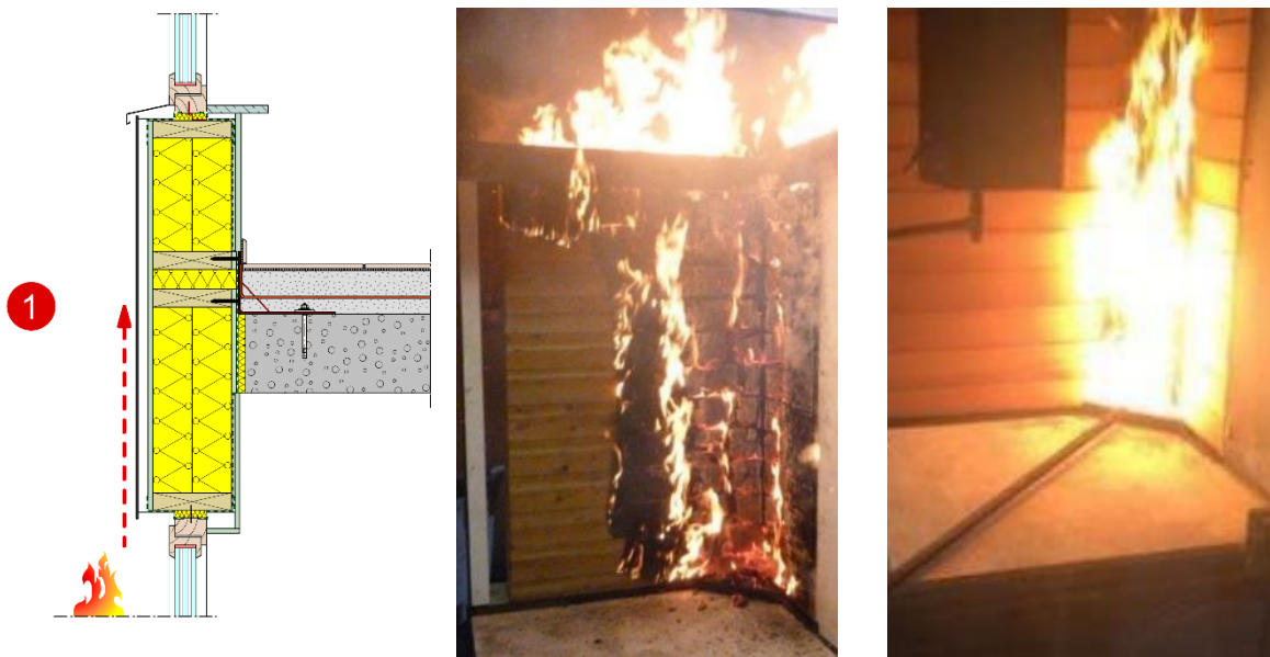
Figure 9 – Fire spread via the surface of the facade cladding (to the left) – Reaction-to-fire tests on wood cladding (centre and right).
