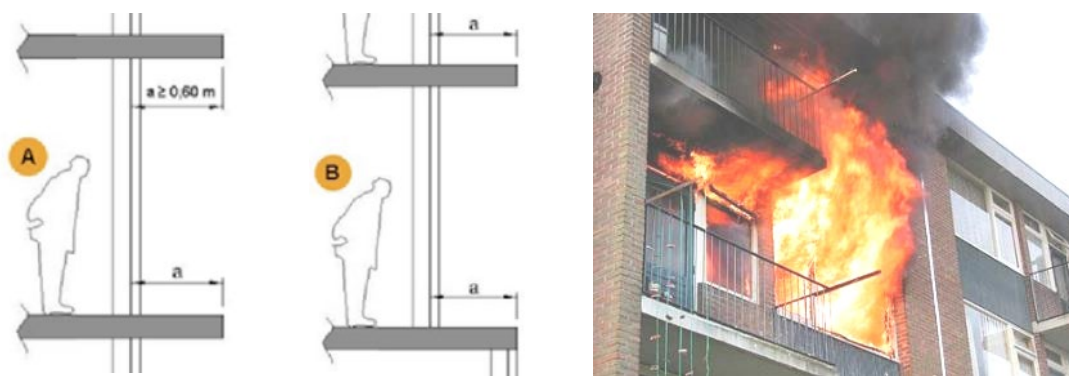
Figure 20 – Horizontal E 60 projection of minimum 60 cm.
