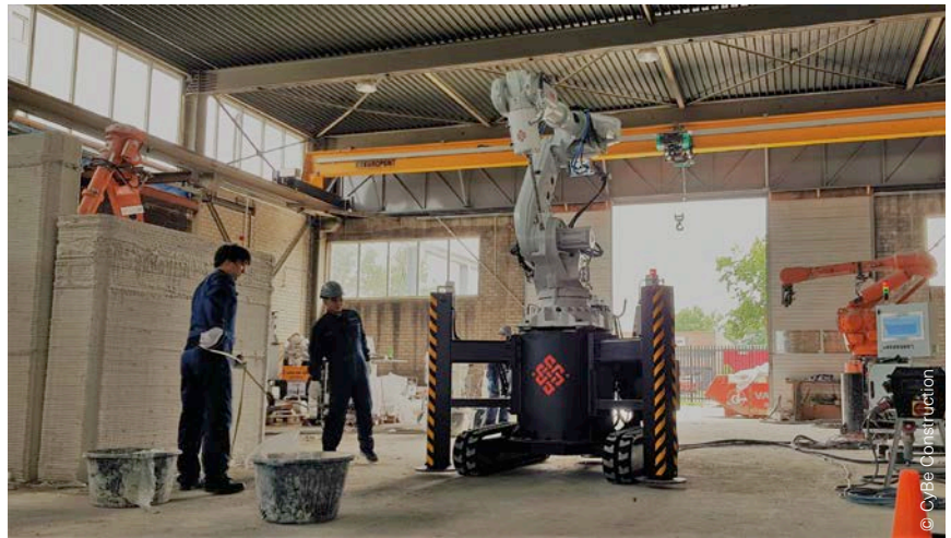
Fig. 43b Imprimantes CyBe R (Robot) et CyBe RC (Robot Crawler) de CyBe Construction – https://cybe.eu/ .
