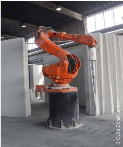
Fig. 43b Imprimantes CyBe R (Robot) et CyBe RC (Robot Crawler) de CyBe Construction – https://cybe.eu/ .
