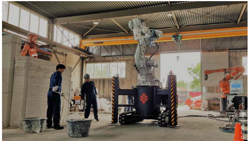
Afb. 43b De printers CyBe R (Robot) en CyBe RC (Robot Crawler) van CyBe Construction – https://cybe.eu/ .
