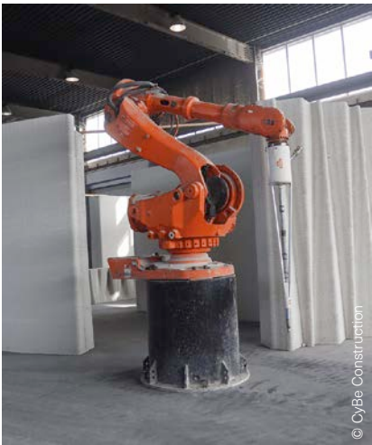
Afb. 43b De printers CyBe R (Robot) en CyBe RC (Robot Crawler) van CyBe Construction – https://cybe.eu/ .
